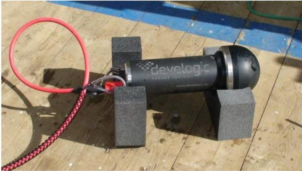
Figure 5. The Develogic surface modem for data transfer to remote user.
