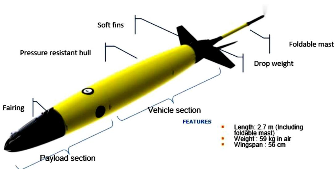
Figure 1. Alseamar's SEA EXPLORER glider system and its two basic components: the vehicle section and the payload section.
