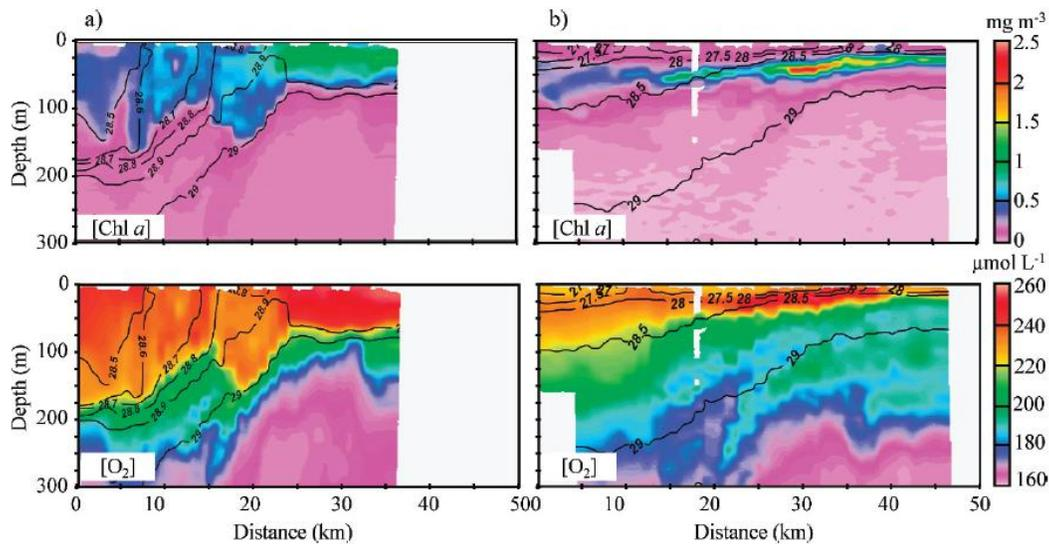
Figure 10. Chl-*a* concentration and DO content glider data along its transect (after Niewiadomska et al., 2008).
