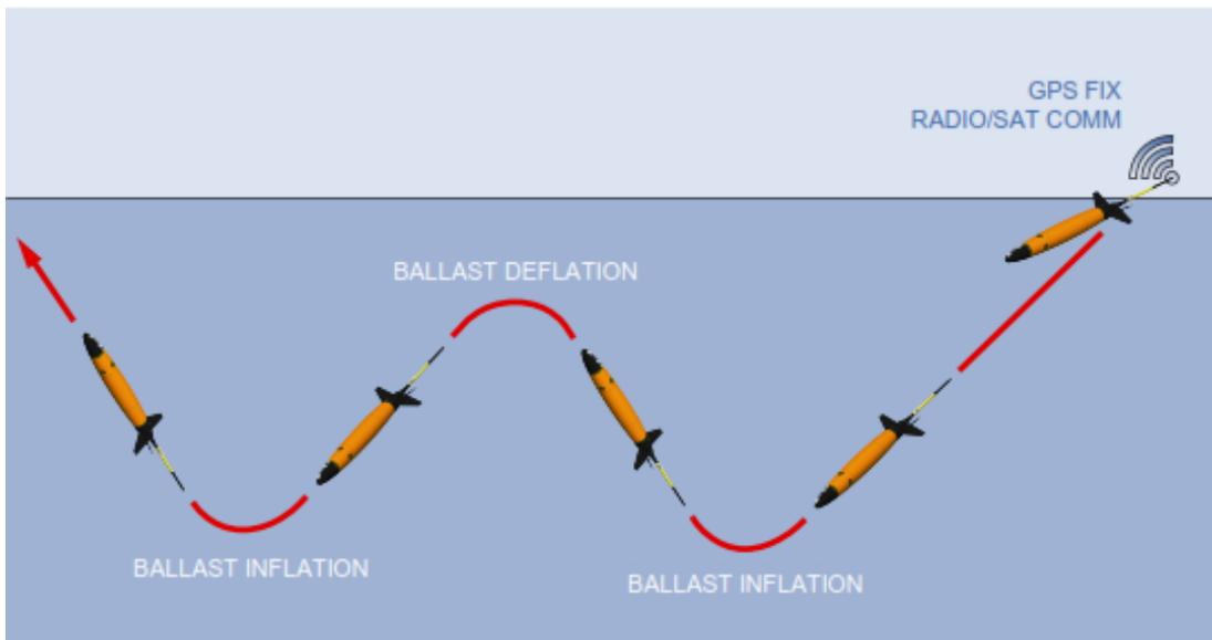
Figure 3. Glider underwater operation.
