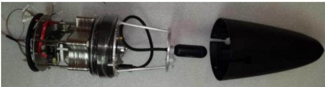
Figure 4. Alseamar's passive acoustic monitoring sensor.
