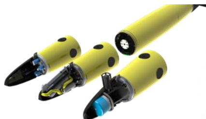
Figure 2. The Modular Seafloor Lander (MSL) and its components and configuration.
